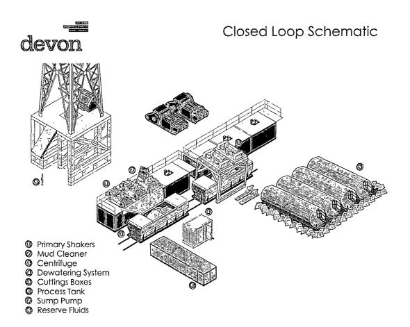
Centrifuges: The centrifuges can be utilized depending on the well's anticipated solids volume. One or two centrifuges can be used depending on the well geometry or depth of well. The centrifuges are sized to maintain low gravity solids at 5% or below. They may or may not need a dewatering system to enhance the removal rates. The centrifuges can make a cut point of 8-10 microns depending on bowl speed, feed rate, solids loading and other factors.
