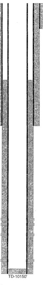
17-1/2" hole @ 1002' 13-3/8" csg @ 1002' w/ 950sx-TOC-Surf-Circ
