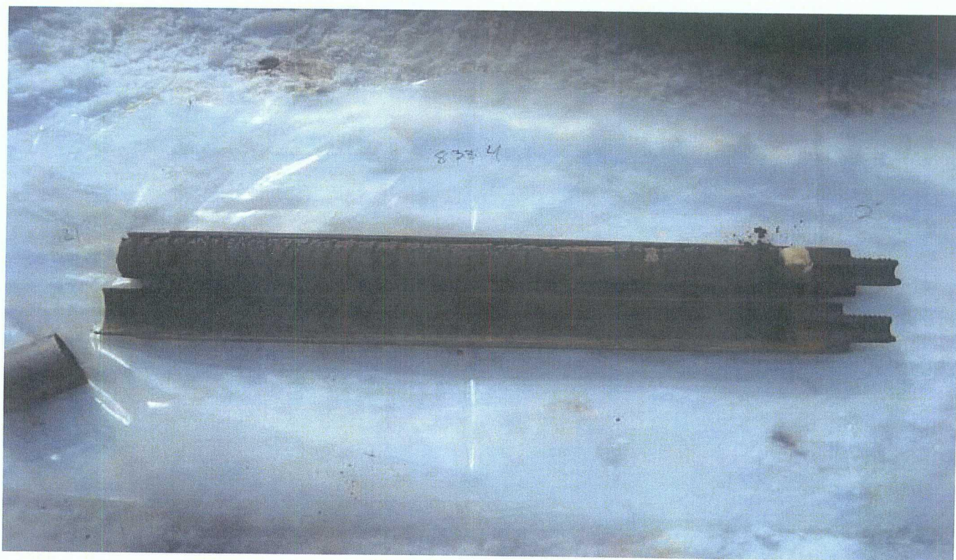
PHOTO 12. 2.5" SAMPLER WITH CUTTINGS FROM 2 TO 4 FT BGS AT SAMPLE LOCATION 8334.
