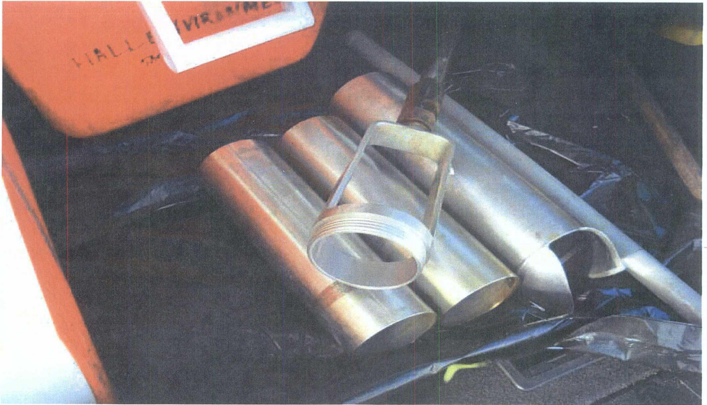
PHOTO 7. STAINLESS STEEL AUGER WITH SLEEVES USED TO COLLECT ZOI SAMPLES.
