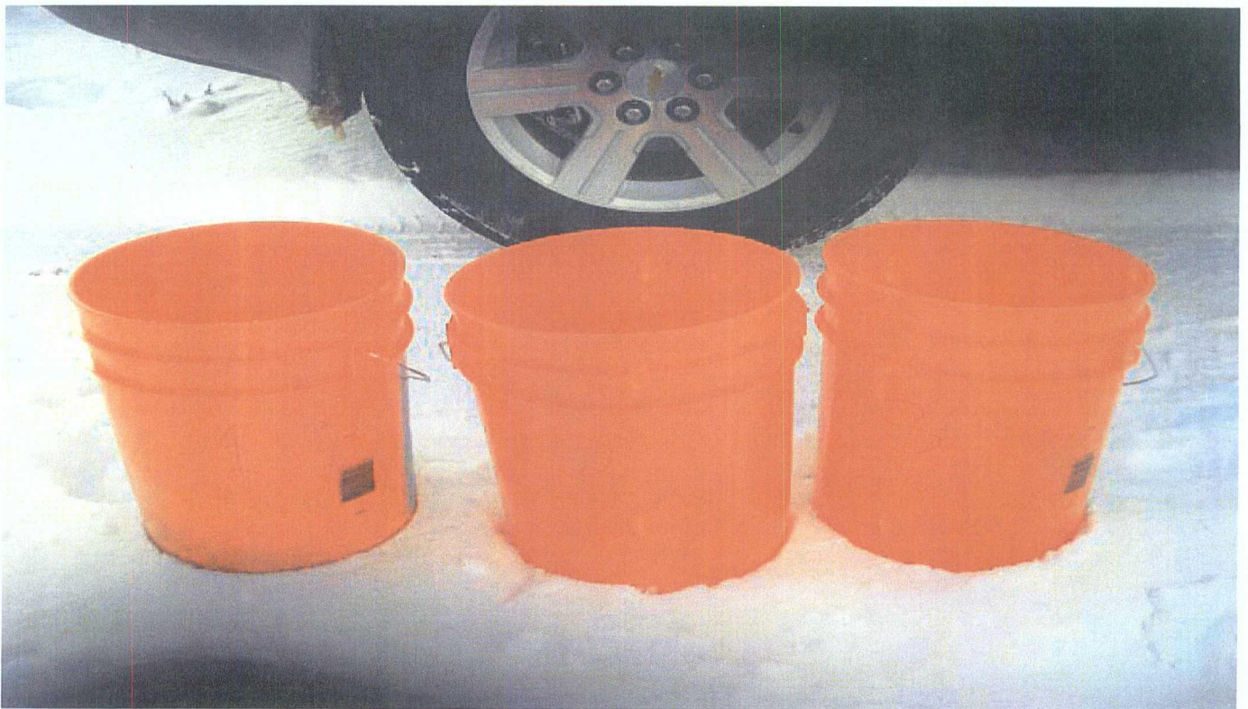
PHOTO 8. DECON STATION, ONE WASH WITH SIMPLE GREEN, TWO RINSE (DISTILLED WATER).
