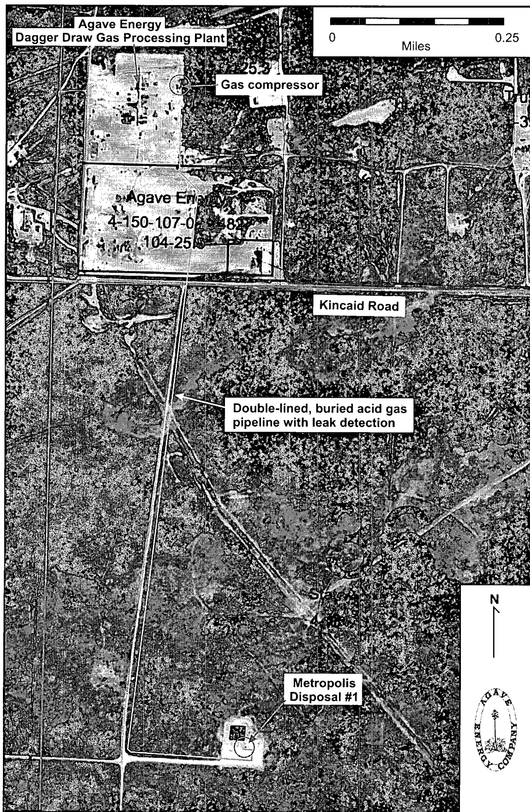
Map 2: General Diagram of Agave Dagger Draw Gas Plant and Location of Pipeline Connecting the Plant with the Metropolis Disposal #1 Well
