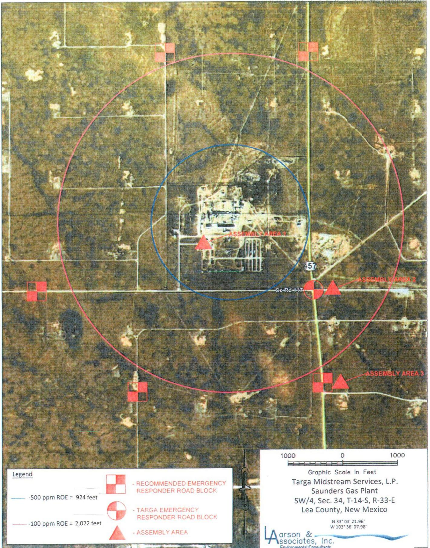
Figure 2 - Radius Of Exposure
