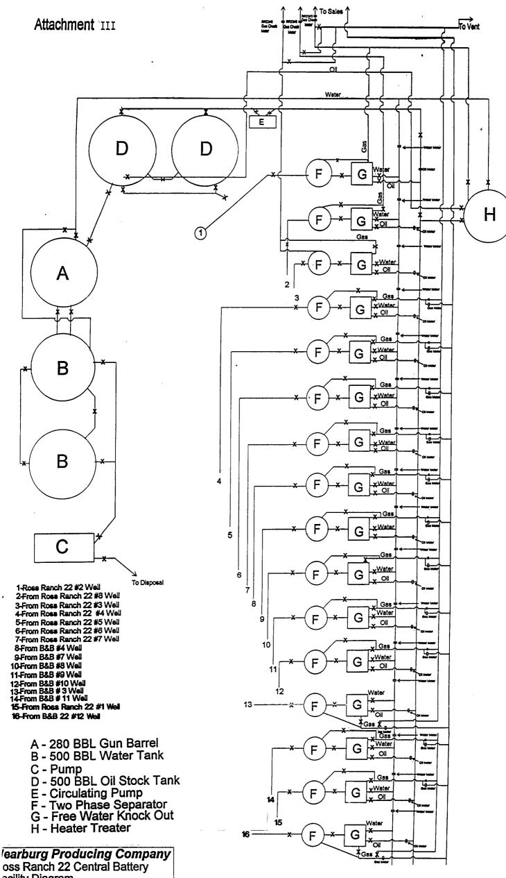
oss Ranch 22 Central Battery acility Diagram 980' FNL & 660' FWL nit E. Section 22, T19S, R25E
