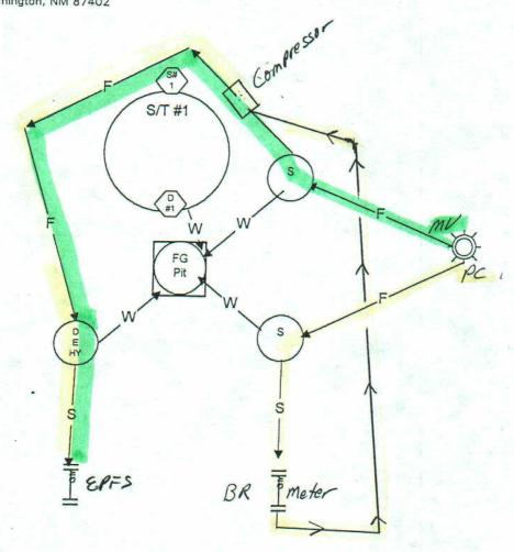
Attachment to the Site Facility Diagram - Lease NM General sealing of valves. Sales by tank gauging PRODUCTION PHASE: All drain valves and all sales valves are sealed closed.
