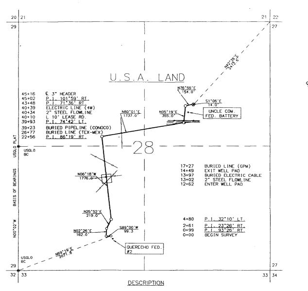
A STRIP OF LAND 50.0 FEET WIDE, 4516.0 FEET OR 0.855 MILES IN LENGTH AND BEING 25.0 FEET LEFT AND RIGHT OF THE ABOVE CENTERLINE SURVEY.
