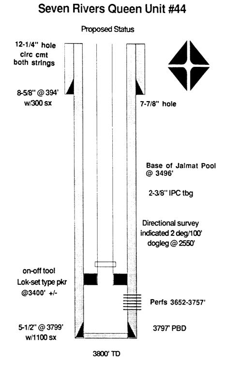
ARCO OIL & GAS COMPANY APPLICATION TO EXPAND SRQU WATERFLOOD PROJECT WELL #44: LANGLIE MATTIX (SR/QN) POOL LOC: 660'FNL & 660'FWL, SEC 2, T23S, R36E, LEA CO. COMPLETED 5/58 AS AN OIL PRODUCER.
