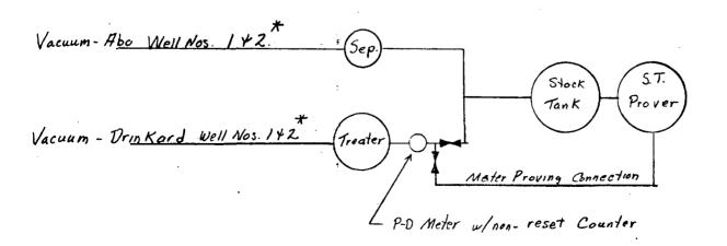
\* No separate testing facilities, two wells each zone, one well will be shut-in while testing.
