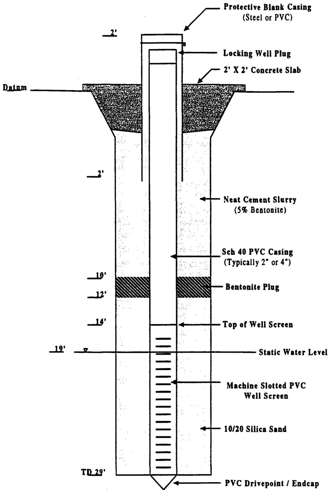
Figure 1: Typical Well Diagram
