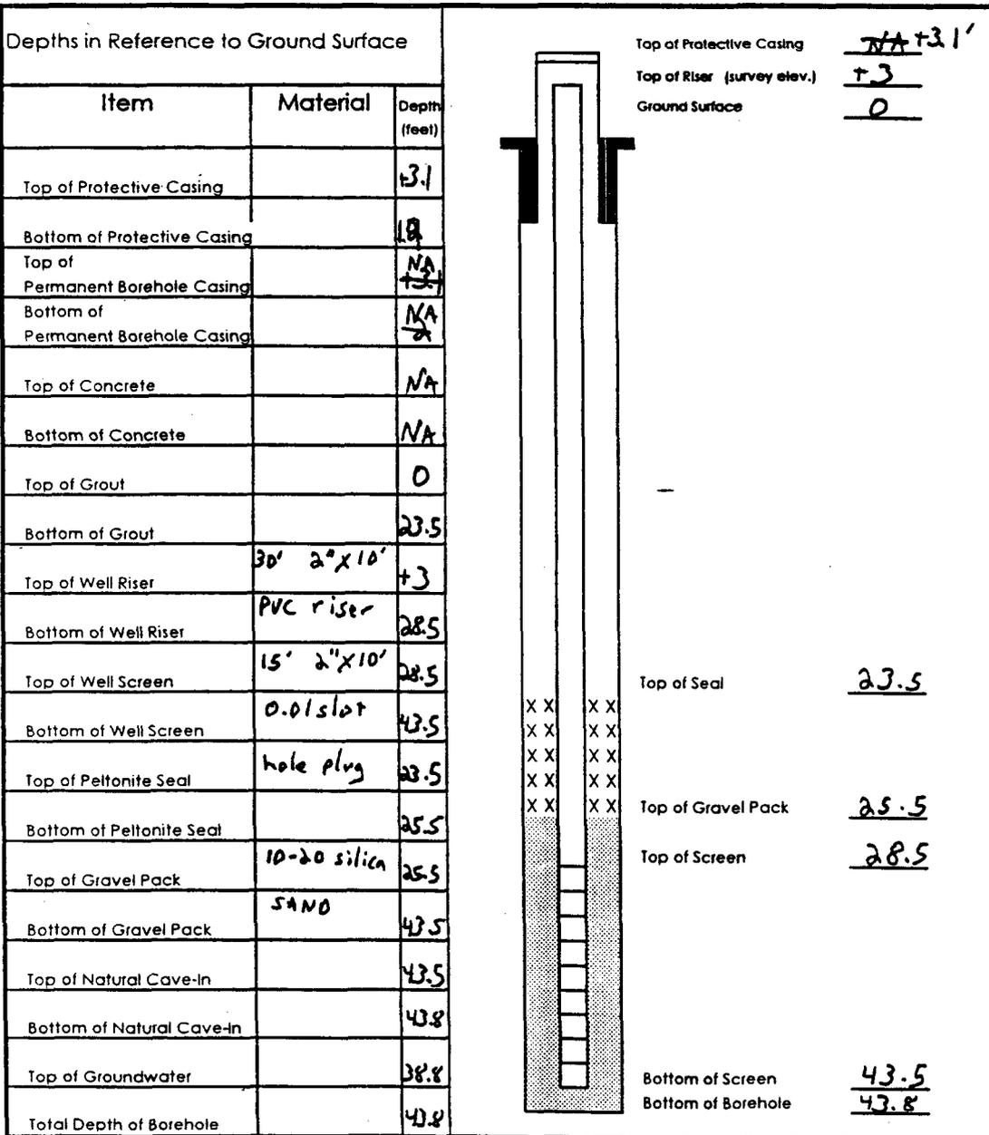
Comments Set well @ 43.5' BGS. Hydrate seal w/ 10 gal potable water. Padlock & locking wellcap on well. Well completed
