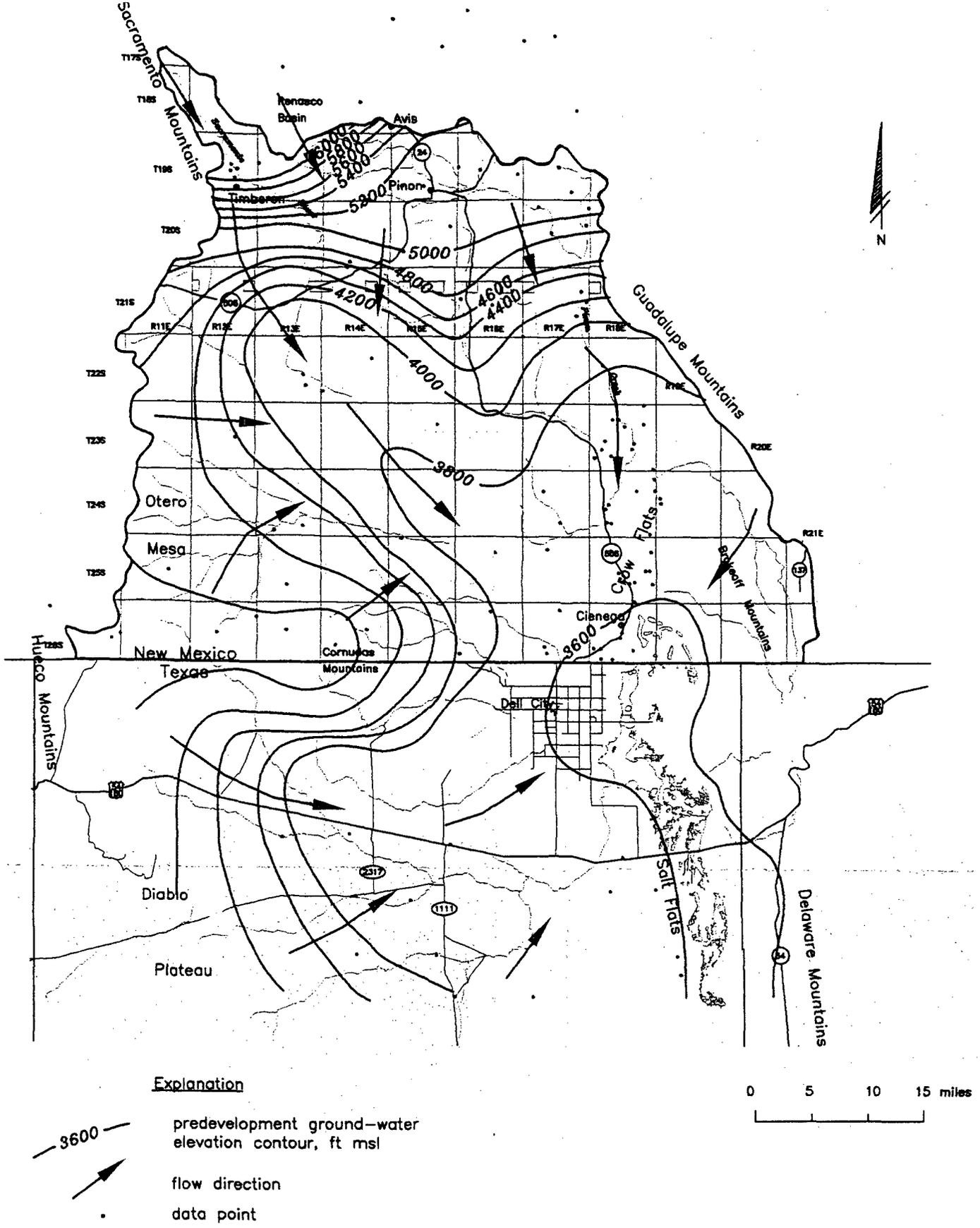
Figure 5. Predevelopment ground-water elevation contours and direction of ground-water flow for the study area.
