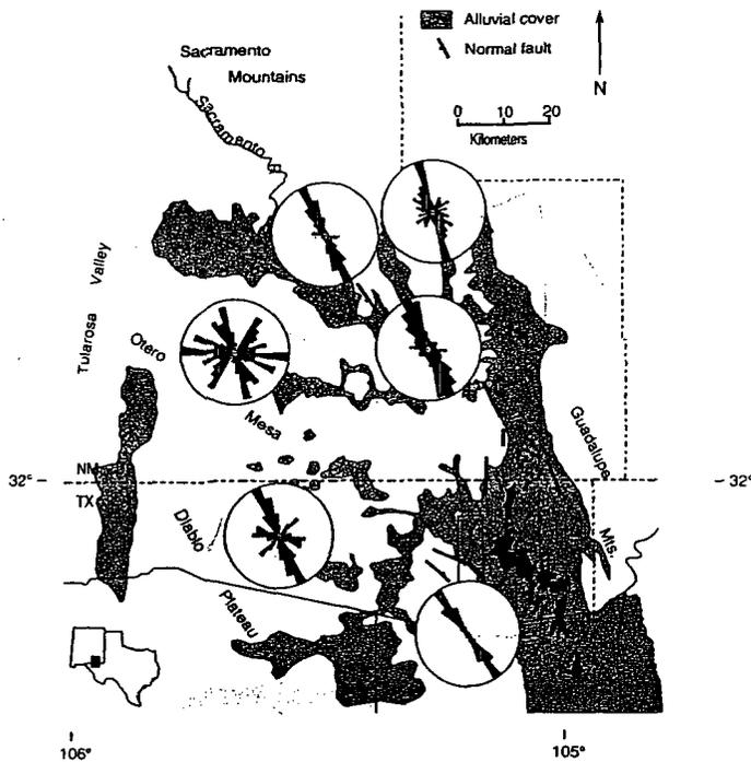
Figure 15. Rose diagrams of fracture orientations. There is a prominent northwest-southeast preferred orientation of fractures across most of region. In Otero Mesa there is no single preferred orientation. Fracture orientation appears to be much less important in regional flow than fracture density.
