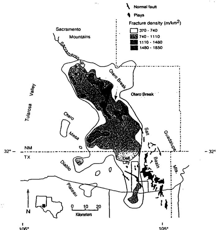
Figure 14. Contour map of fracture density (meters per square kilometer). Note concentration of fractures along Otero Break. Fracture density is least in western Otero Mesa where Yeso Formation crops out. No fractures are mapped in alluvial cover. We hypothesize that fracture distribution is major control of regional ground-water flow.
