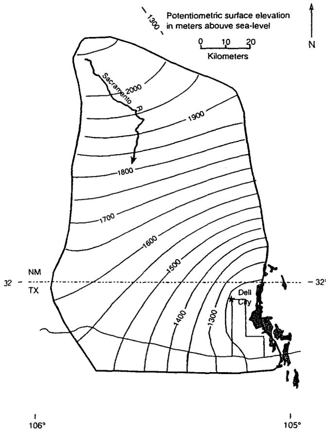
Figure 17. Model-generated potentiometric surface for homogeneous, isotropic transmissivity. By comparison with Figure 9 it is apparent that homogeneous transmissivity is not consistent with the observed hydraulic head distribution, given estimated recharge.
