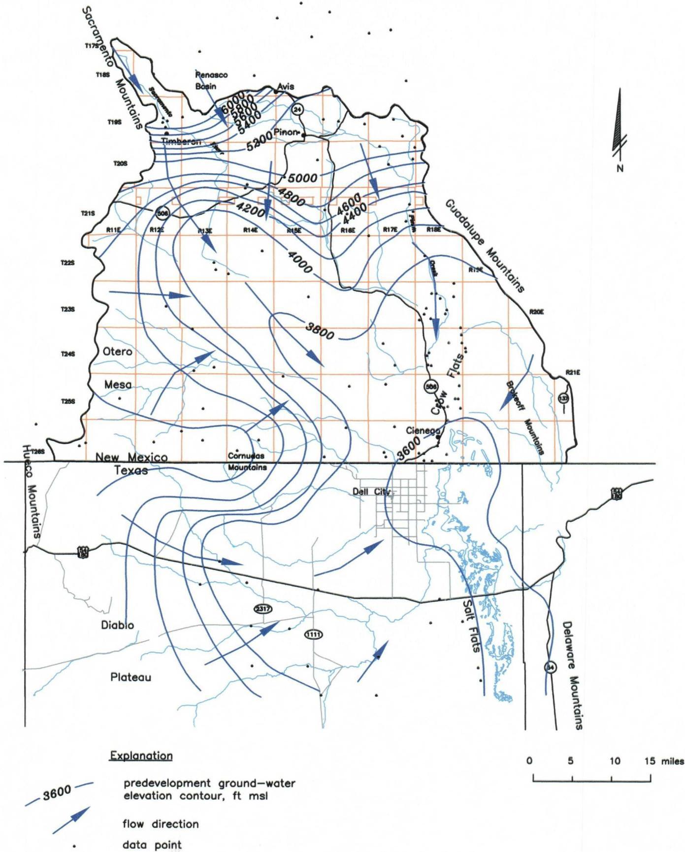
Figure 5. Predevelopment ground-water elevation contours and direction of ground-water flow for the study area.
