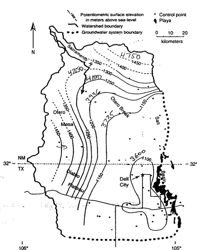
Figure 9. Regional potentiometric surface map. Note low hydraulic gradient in southeastern part of region, and broad, northwest-trending potentiometric trough, coincident with Otero Break. These features correspond to areas of relatively intense fracturing and suggest that fracturing plays a major role in determining ground-water flow in this area. TDS—total dissolved solids.
