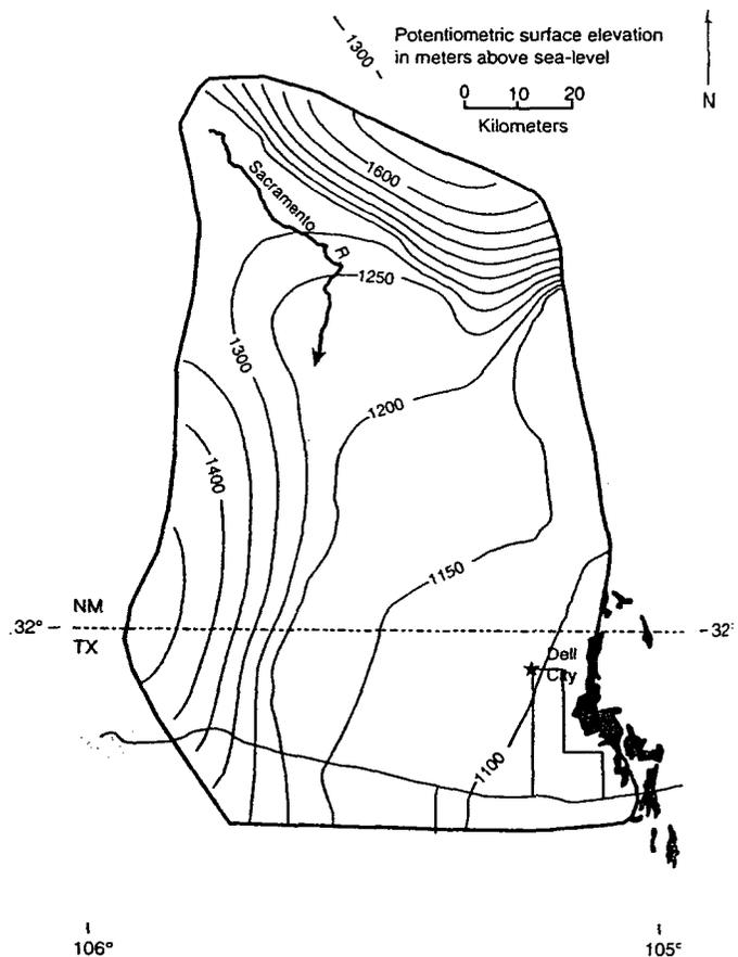
Figure 18. Model-generated potentiometric surface assuming heterogeneous, isotropic transmissivity distribution defined on the basis of fracture density. This transmissivity distribution produces a hydraulic head distribution similar to the observed potentiometric surface. Thus regional potentiometric trends are consistent with a high-transmissivity zone coincident with fracturing along the Otero Break.
