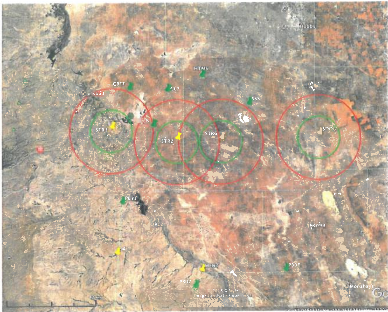
Figure 1. Striker SWD wells seismic station locations and existing NGL-Permian seismic stations (yellow pushpins). Green and red circles around stations show approximate detection levels for ML 1.0 and 1.5, respectively.
