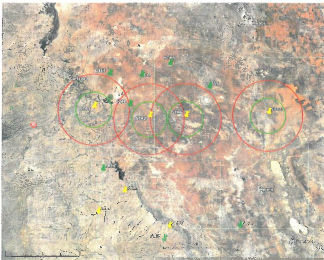
Figure 1. NGL-Permian seismic stations (yellow pushpins). Green and red circles around stations show approximate detection levels for ML 1.0 and 1.5, respectively.
