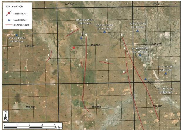
Identified faults in the area of the proposed Independence AGI #1 well and nearby SWD wells included in slip-probability modeling simulations
