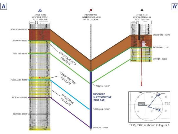
Cross section showing cap rock (Woodford Shale) and porous zones (yellow) identified within the targeted injection interval
