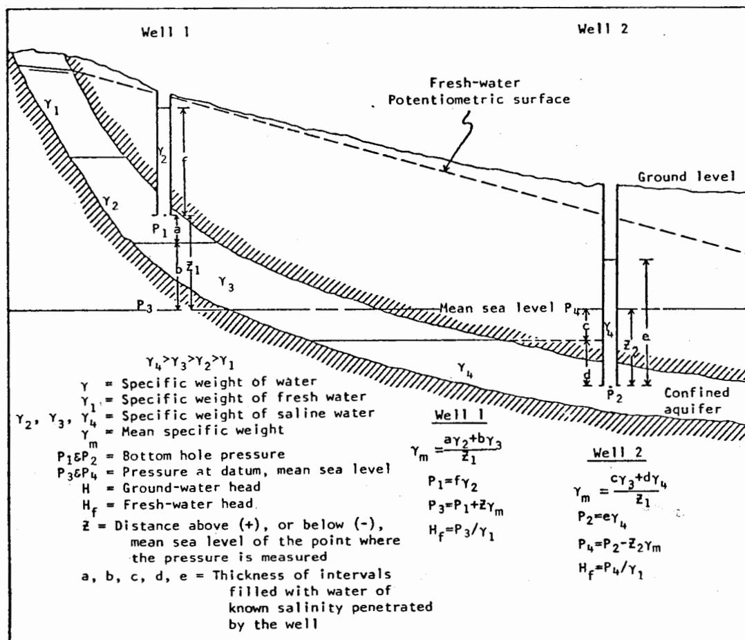
Figure 30.--Diagram showing computation of fresh-water head for wells tapping a confined aquifer containing water of variable density.
