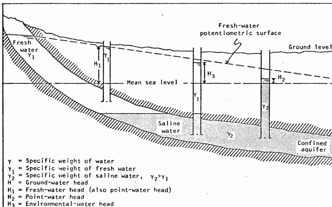
Figure 29.--Diagram showing heads and fresh-water potentiometric surface for confined aquifer containing water of variable density.
