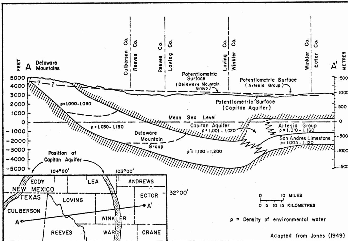
Figure 32.--Diagrammatic profile of Capitan and associated aquifers across western Texas showing pre-oil-discovery potentiometric surfaces and variation in the density of the ground water.
