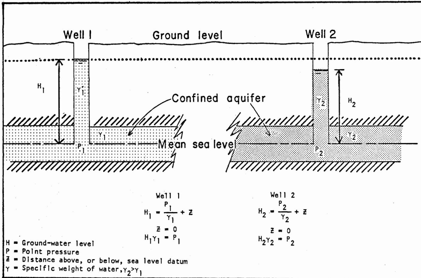
Figure 31.--Diagram showing head relationships in wells tapping a confined aquifer containing water of variable density.
