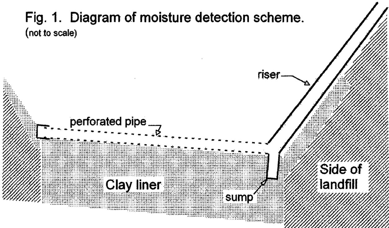
Perforated pipe may be laid within the operations layer or on the clay liner.
