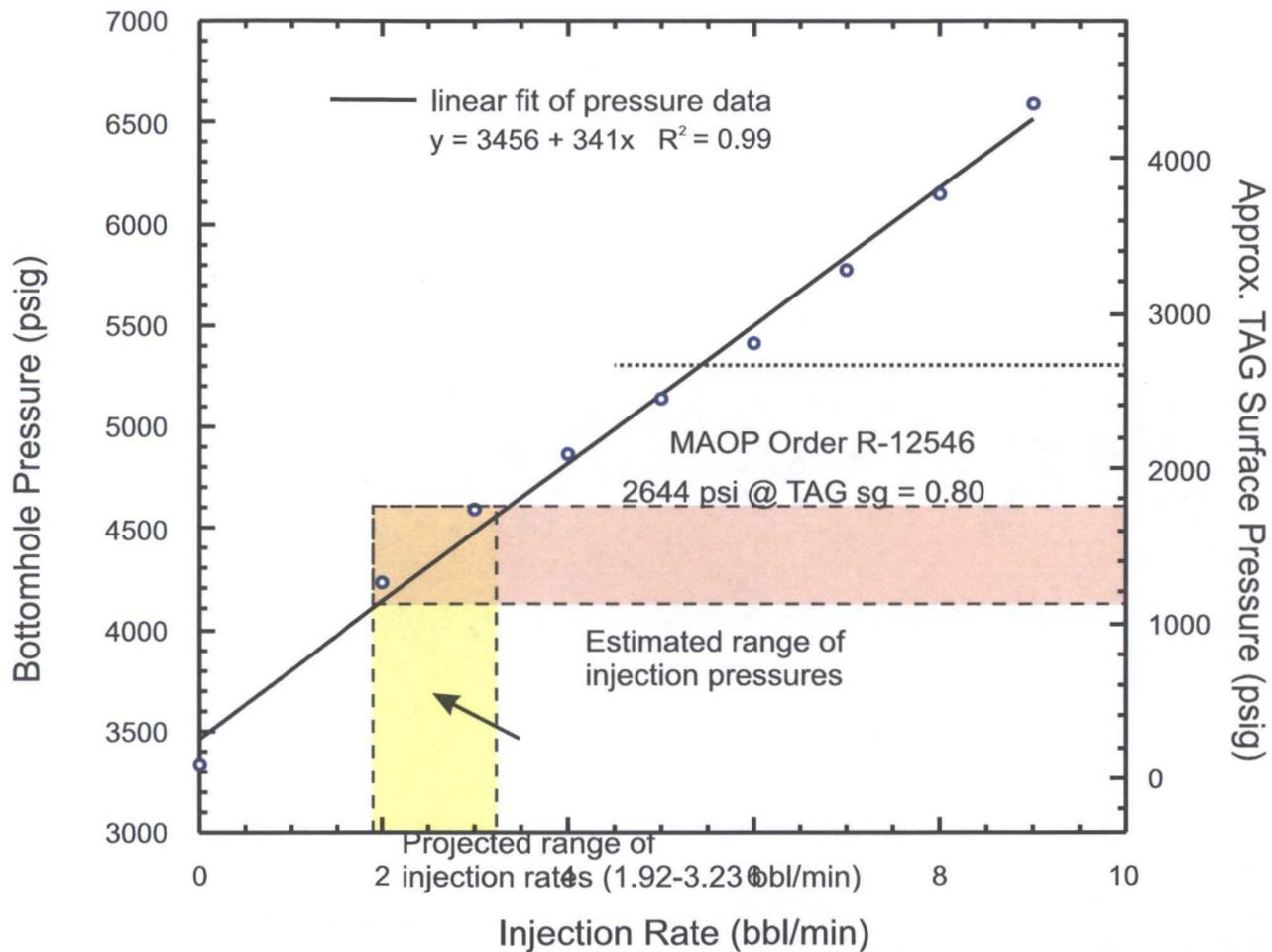
Note: Approx. TAG Surface Pressure is calculated using the initial reservoir pressure (3262 psi) and the ave. specific gravity of TAG ranging from 0.80 to 0.69. Note that during workover in April-May 2012, well Linam AGI #1 went on vacuum while killed, indicating an underpressured reservoir even after almost three years of operation at Linam AGI #1.
