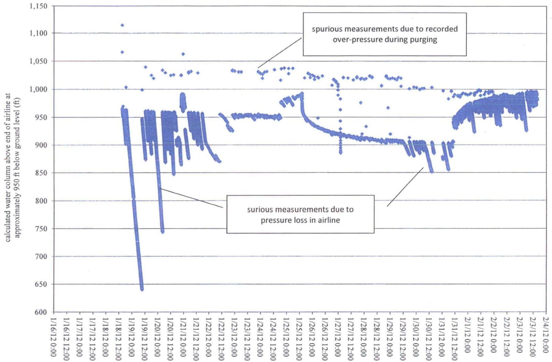
Figure 3A. Depth to water in Well 45-7 during closed-loop test.
