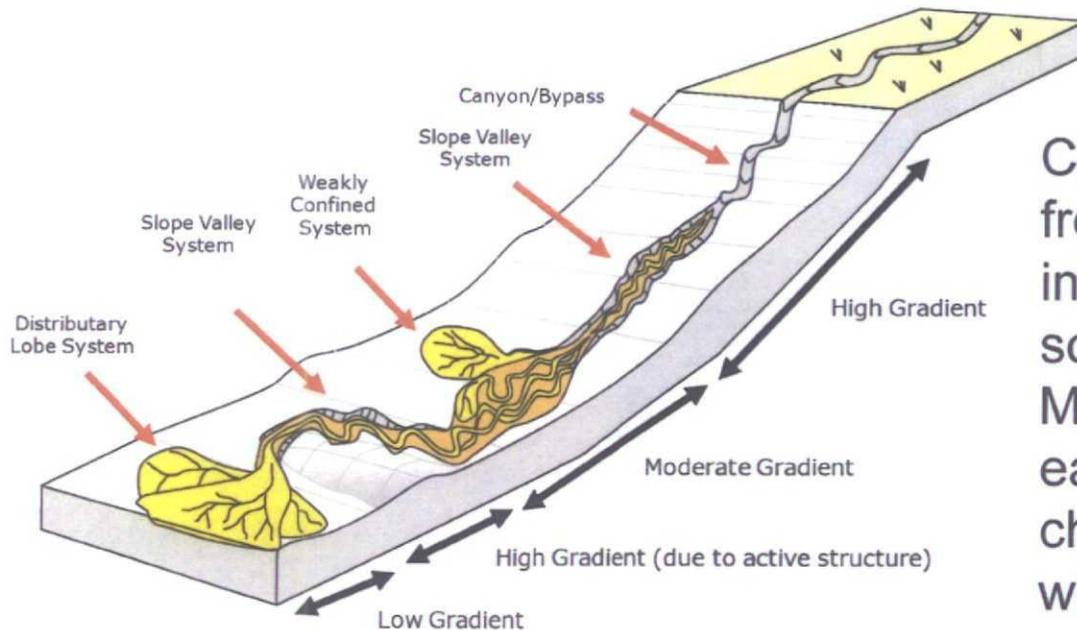
Channel system sourced from the north and grades into a fan system to the south in the basin. Mitigate risk by drilling east-west to dissect axis of channel. Axis of channel will have better porosity.
