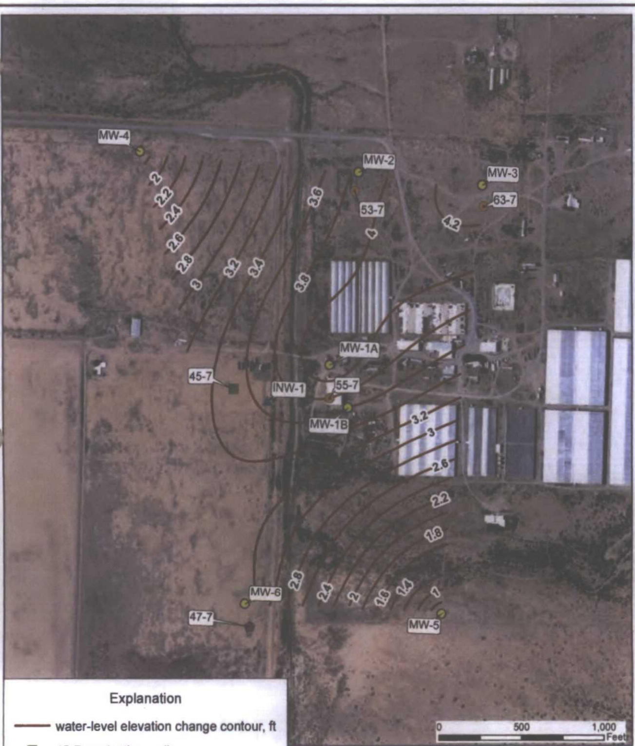
Figure 16. Water-level elevation change in shallow monitoring wells (MW- wells) between December 09, 10, and 11, 2013 (prior to beginning of geothermal operations) and May 11, 2014, Cyrg Energy Lightning Dock Geothermal project. Contour values in feet. Positive value indicates water-level rise.
