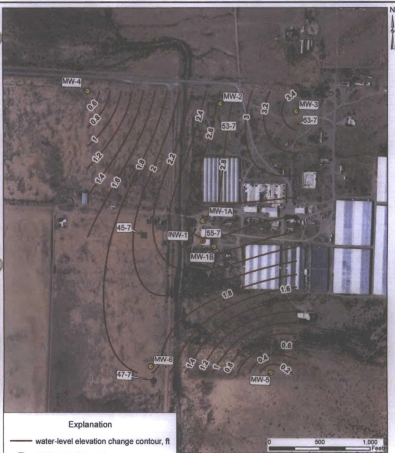
Figure 12. Water-level elevation change in shallow monitoring wells (MW- wells) between December 09, 10, and 11, 2013 (prior to beginning of geothermal operations) and January 27, 2014, Cyrrq Energy Lightning Dock Geothermal project. Contour values in feet. Positive value indicates water-level rise.
