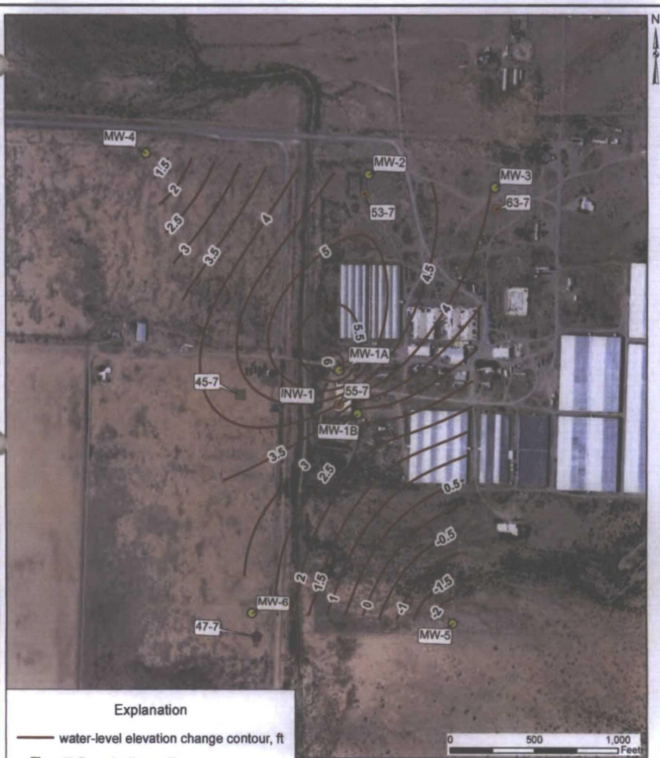
Figure 17. Water-level elevation change in shallow monitoring wells (MW- wells) between December 09, 10, and 11, 2013 (prior to beginning of geothermal operations) and June 19, 2014, Cyrg Energy Lightning Dock Geothermal project. Contour values in feet. Positive value indicates water-level rise.
