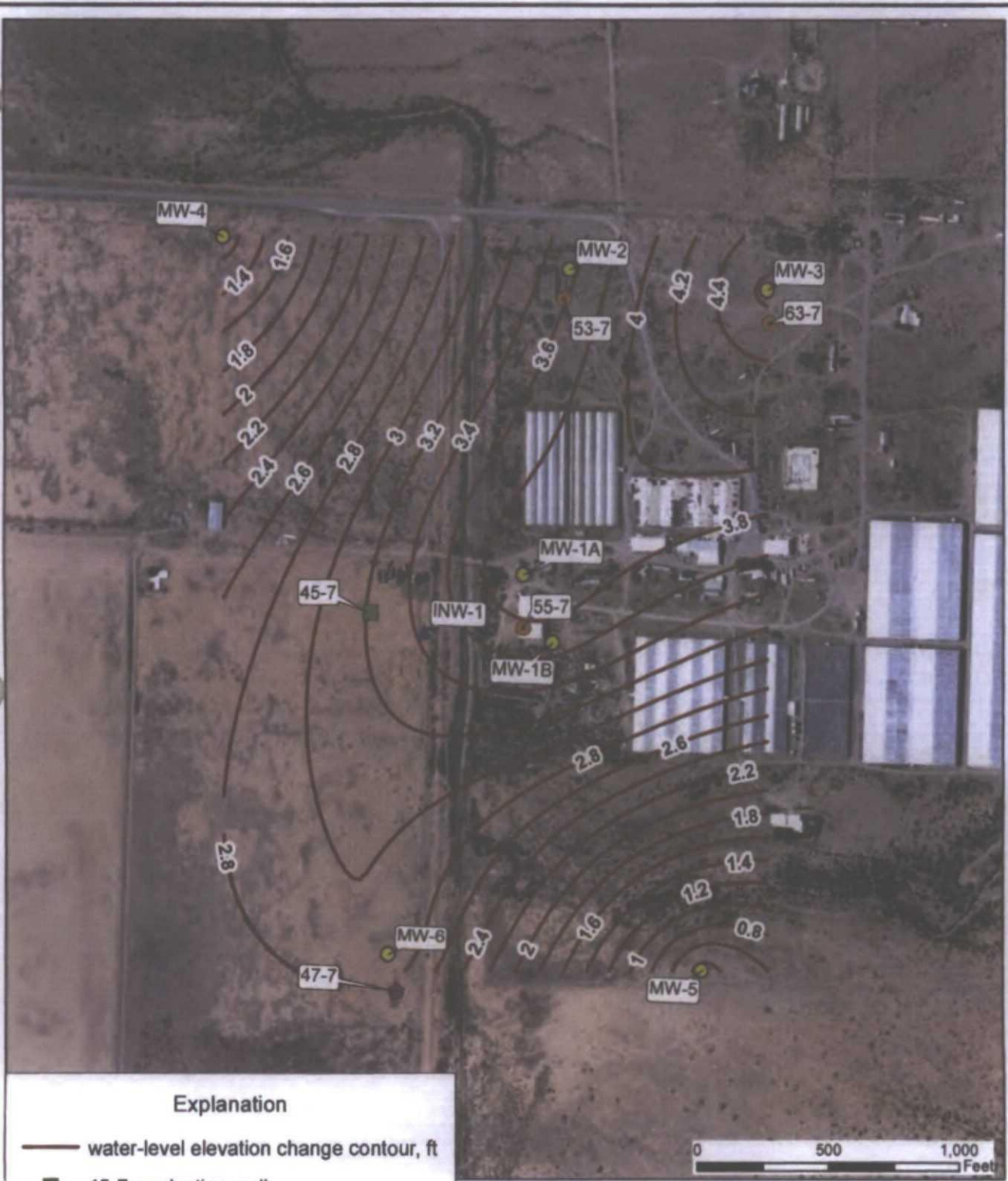
Figure 14. Water-level elevation change in shallow monitoring wells (MW- wells) between December 09, 10, and 11, 2013 (prior to beginning of geothermal operations) and March 17, 2014, Cyrg Energy Lightning Dock Geothermal project. Contour values in feet. Positive value indicates water-level rise.
