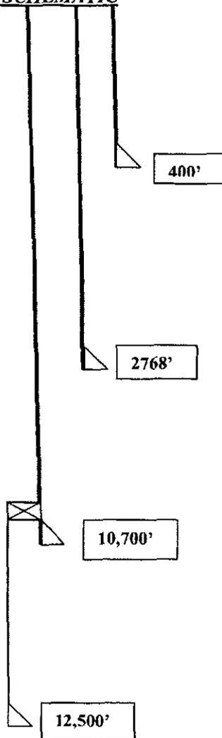
4.5" 13.5# P110 liner, 6.15" hole, cemented to top of liner w/ 295 sacks, circulated 55 sacks off of liner top. Top of liner is 10,277'
