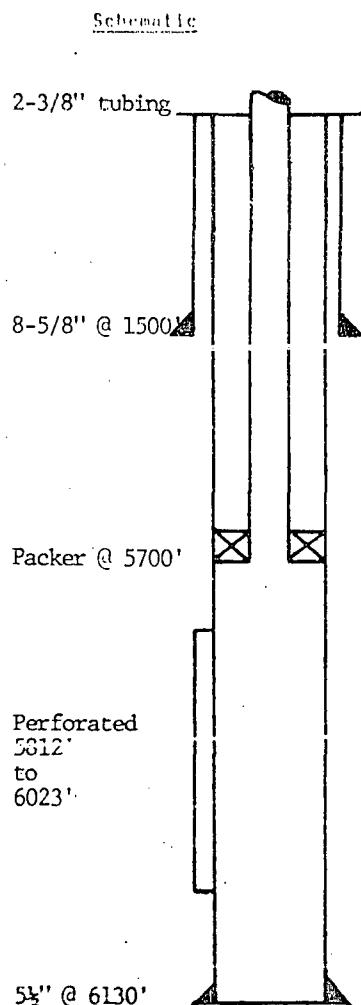
SchematicIntubular DataSurface Casing
