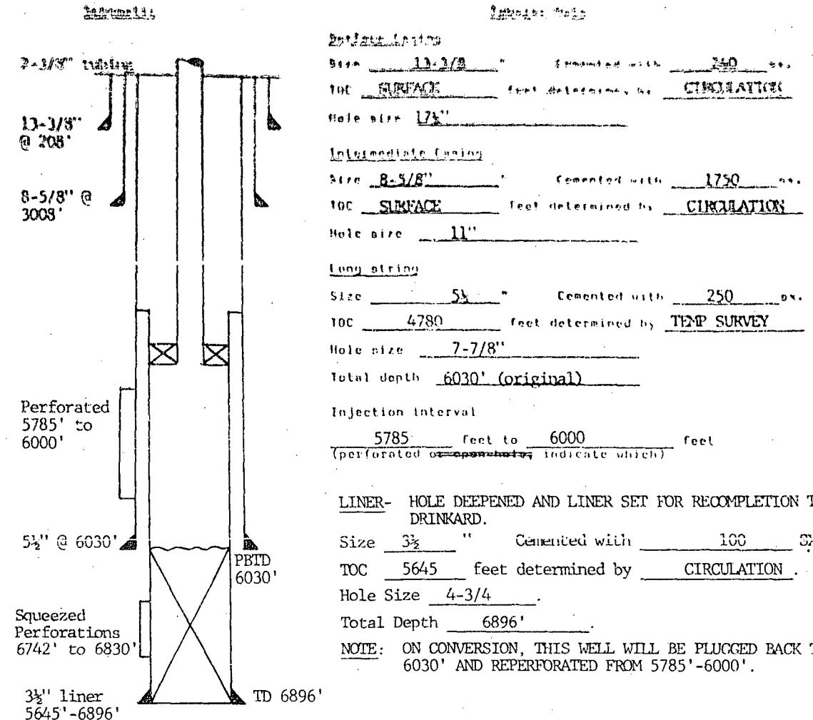
Tubing size 2-3/8" lined with PLASTIC (material) set in a
