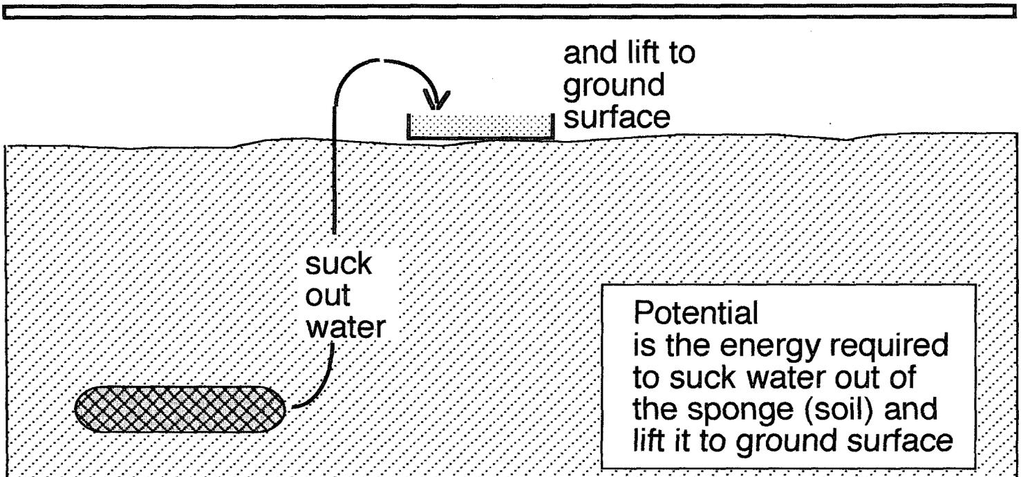
Fig. 2. Schematic diagrams of suction and potential.
