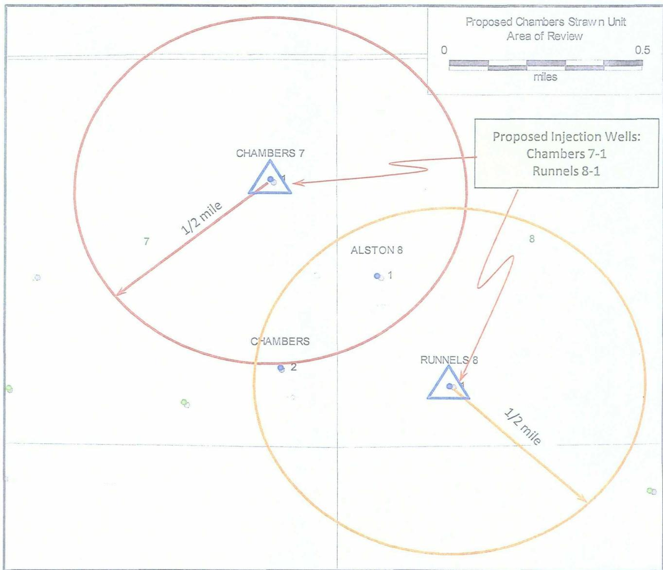
Two wells will be converted to injection, the Chambers 7 # 1 and the Runnels 8 #1. There are two other wells within the area of review, the Alston 8 #1 and the Chambers #2. All pertinent well data is on the table of review. Wellbore schematics are attached showing each proposed injectors as presently configured and as it will be configured for injection service.
