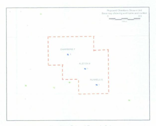
We propose Chambers 7-1 and Runnels 8-1 be converted to water injection service.
