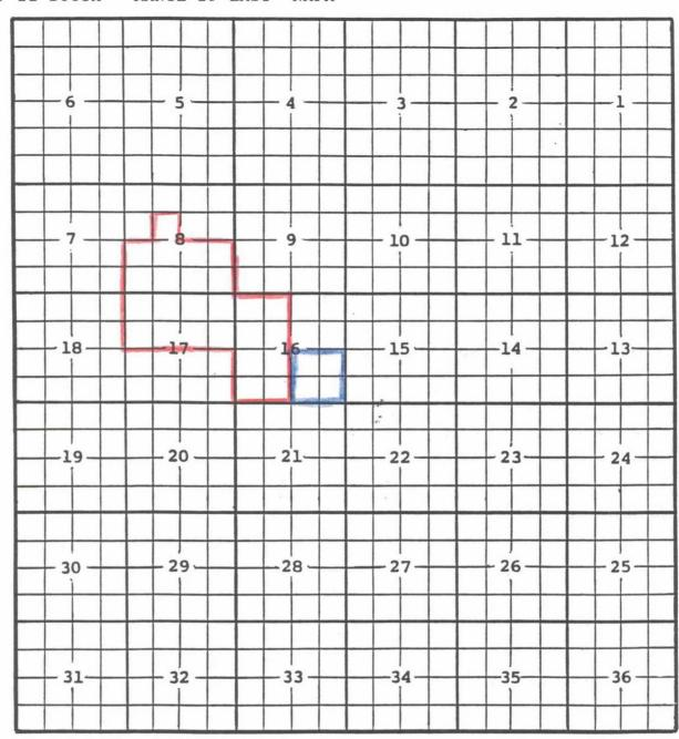
PURPOSE: One completed oil well capable of producing. Enron Oil & Gas Co., Big Eddy Unit No.132 Unit J, Sec.16, T.21S., R.29E., NMPM. Completed 4-15-94 in the Delaware formation. Top of perforations are at 5675 feet.
