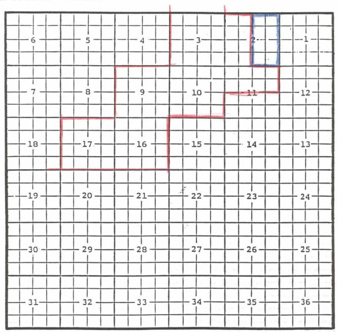
PURPOSE: One completed well capable of producing. Nearburg Prod. Co., Big Walt 2 State No.2 Unit J, Sec.2, T.22S., R.24E., NMPM. Completed 4-11-94 in the Upper Penn formation. Top of perforations are at 7862 feet.
