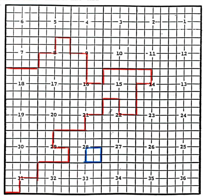
PURPOSE: One completed oil well capable of producing. Yates Pet. Tackitt AOT No.1 Unit J, Sec.28 T.19S., R.25E., NMPM. Completed 10-26-94, in the Upper Penn formation. Top of perforations are at 7606 feet.
