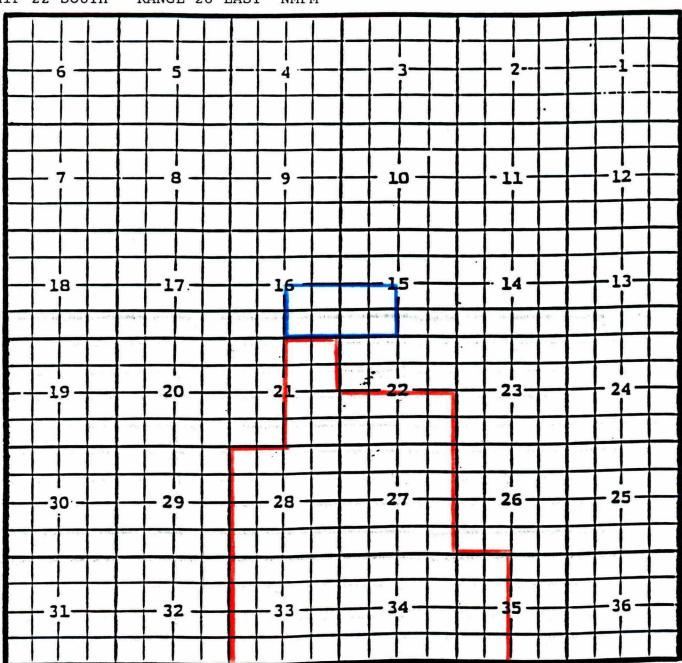
PURPOSE: One completed gas well capable of producing. Dinero Oper. Co., Big Chief Com. No.4 Unit N, Sec.15 T.22S., R.28E., NMPM. Completed 8-15-94 in the Atoka formation. Top of perforations are at 11442 feet.
