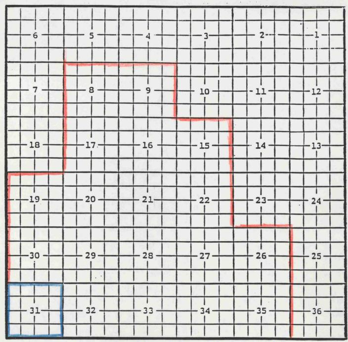
PURPOSE: One completed gas well capable of producing. Texaco Exploration and Production Co., White City "31" Federal #1 Unit G, Sec. 31, T.24S., R.26E., NMPM. Completed 4-16-95 in the Penn. formation. Top of perforations are at 11326 feet.
