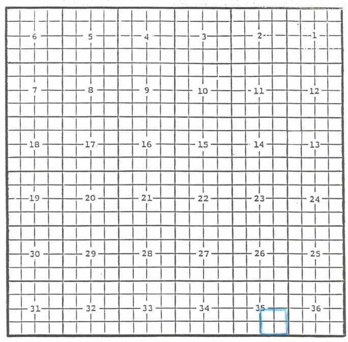
PURPOSE: One completed oil well capable of producing. Hallwood Petroleum Inc., Harkey 35 State #1 Unit J, Sec. 35, T.24., R.27E., NMPM. Completed 02-14-95 in the Bone Spring formation. Top of perforations are at 8210 feet.
