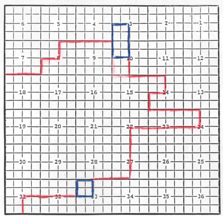
PURPOSE: One completed oil well capable of producing. Mewbourne Oil Company, State "B" Com. #2 Unit D, Sec.33, T.19S.,R.25E., NMPM. Completed 11-11-95 in the Upper Penn. formation. Top of perforations are at 7690 feet.
