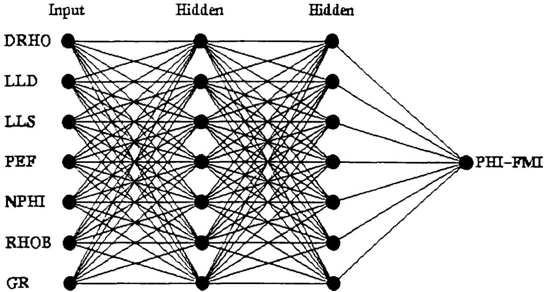
**Figure 2.** Fully connected 4-layer Neural Network architecture used in this study. The input layer is comprised of the seven selected traditional wireline logs. Each neuron is linked to each neuron in the next layer making this a fully connected network. Each connection generates one weight, for a total of 105 weights using this architecture.
