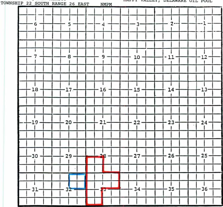
PURPOSE: One completed oil well capable of producing. Louis Dreyfuss Natural Gas Corp., "EV" State #3 Unit A, Sec.32, T-22-S, R-26-E, NMPM. Completed 2/96 in the Delaware formation. Top of perforations are at 4190 feet.
