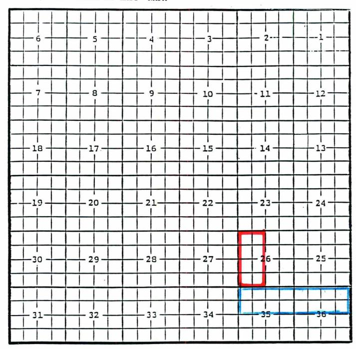
PURPOSE: One completed gas well capable of producing. Yates Petroleum Corp., Cedro "APG" St. Com. #1 Sec.36 T-17-S, R-30-E, NMPM UNIT C Completed 2/96 in the Atoka formation. Top of perforations are at 10853 feet.
