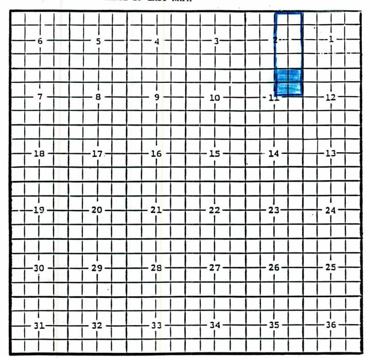
PURPOSE: One completed oil well capable of producing. Santa Fe Energy Resources Inc., Corral Fly "11" State #1 Unit A, Sec. 11, T-25-S, R-29-E, NMPM. Completed 3/96 in the Delware formation. Top of perforations are at 5364 feet.
