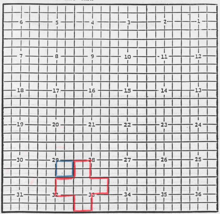
PURPOSE: One completed oil well capable of producing. Louis Dreyfus Natural Gas Corp., Happy Valley "29" #4 Unit P, Sec. 29, T.22S., R26E., NMPM Completed 6-01-96 in the Delaware formation. Top of perforations are at 2500 feet.
