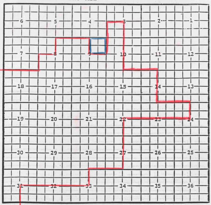
PURPOSE: One completed oil well capable of producing. Yates Petroleum Corp., Patrick "API" #3 Unit A, Sec.9, T.19S., R.25E., NMPM. Completed 6-01-96 in the Upper Penn. formation. Top of perforations are at 7744 feet.
