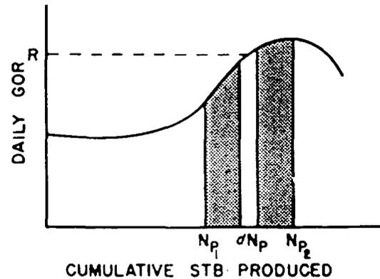
Fig. 3.12. Typical daily gas-oil ratio curve for a dissolved gas drive reservoir.
