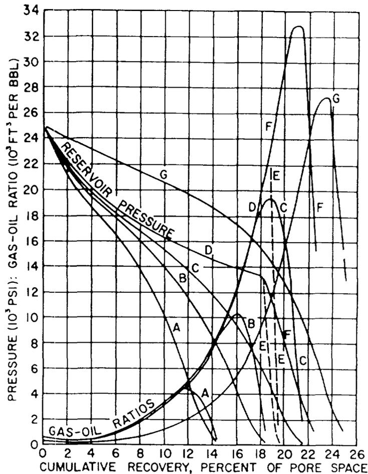
Fig. 7.17. Theoretical pressure and gas-oil ratio histories of gas drive reservoirs subjected to various gas return programs. (A)  $r = 0$ ,  $m = 0$ ; (B)  $r = 0.66$ ,  $m = 0$ ; (C)  $r = 0.80$ ,  $m = 0$ ; (D)  $r = 1.00$  up to  $R = 20,000$  SCF/STB,  $m = 0$ ; (E) Continuation of D with  $r = 0$ ; (F) Continuation of D with  $r = 0.80$ ; (G) Initial gas cap,  $m = 0.50$ ,  $r = 0.80$ . (After Muskat, *Oil and Gas Journal*, Vol. 47, No. 48, p. 89.)
