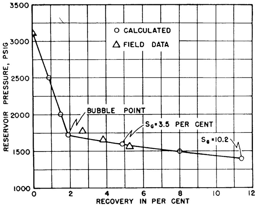
Fig. 3.9. Material balance calculations and performance, Canyon Reef reservoir, Kelly-Snyder Field.
