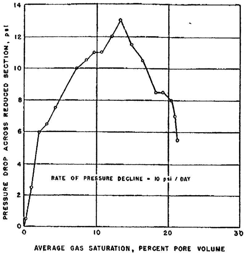
FIG. 7 - PRESSURE DROP PERFORMANCE ACROSS REDUCED SECTION OF CORBY SHELLSTONE.
