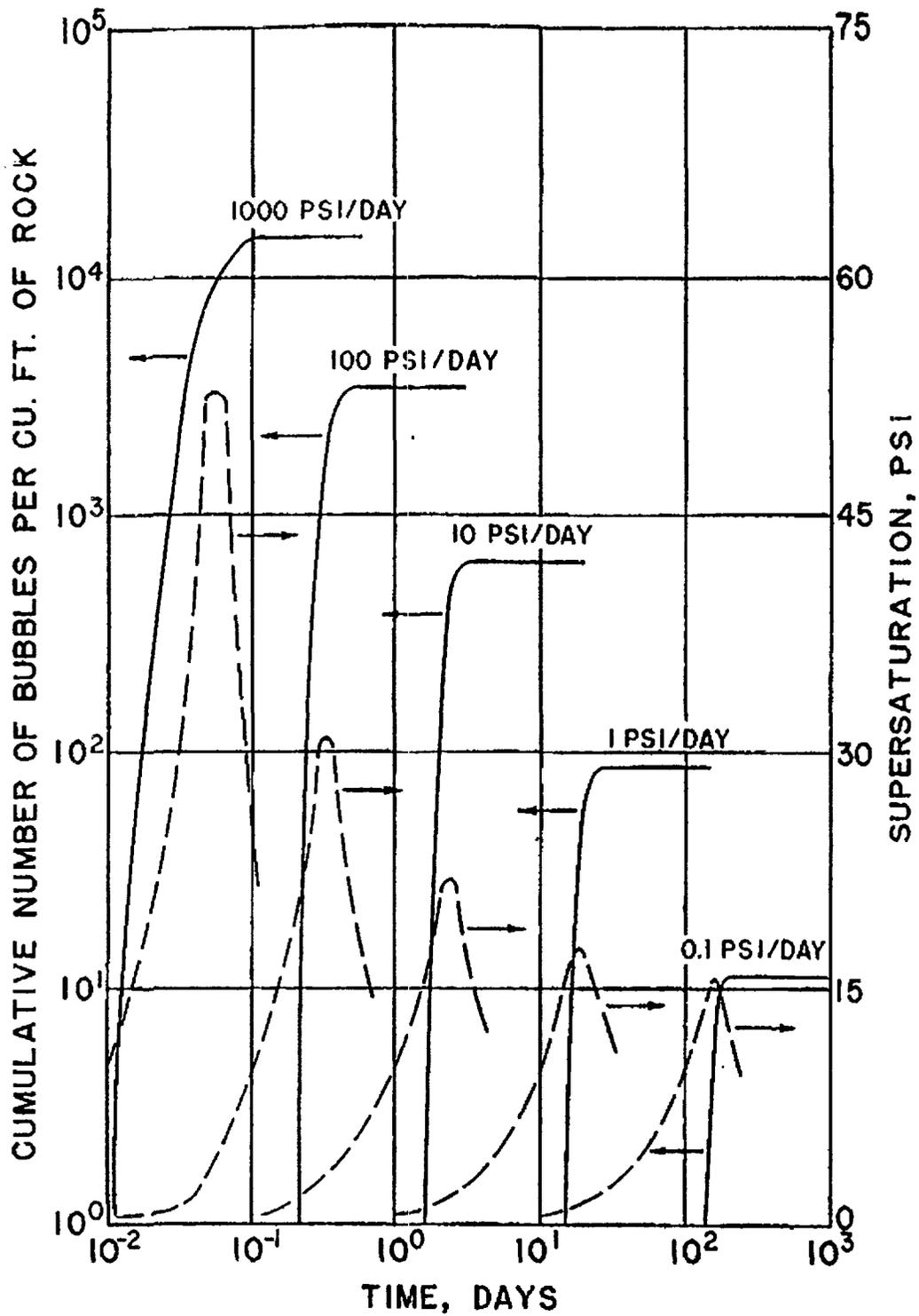
FIG. 3 - CALCULATED SUPERSATURATION AND BUBBLE FORMATION ASSOCIATED WITH VARIOUS RATES OF PRESSURE DECLINE.
