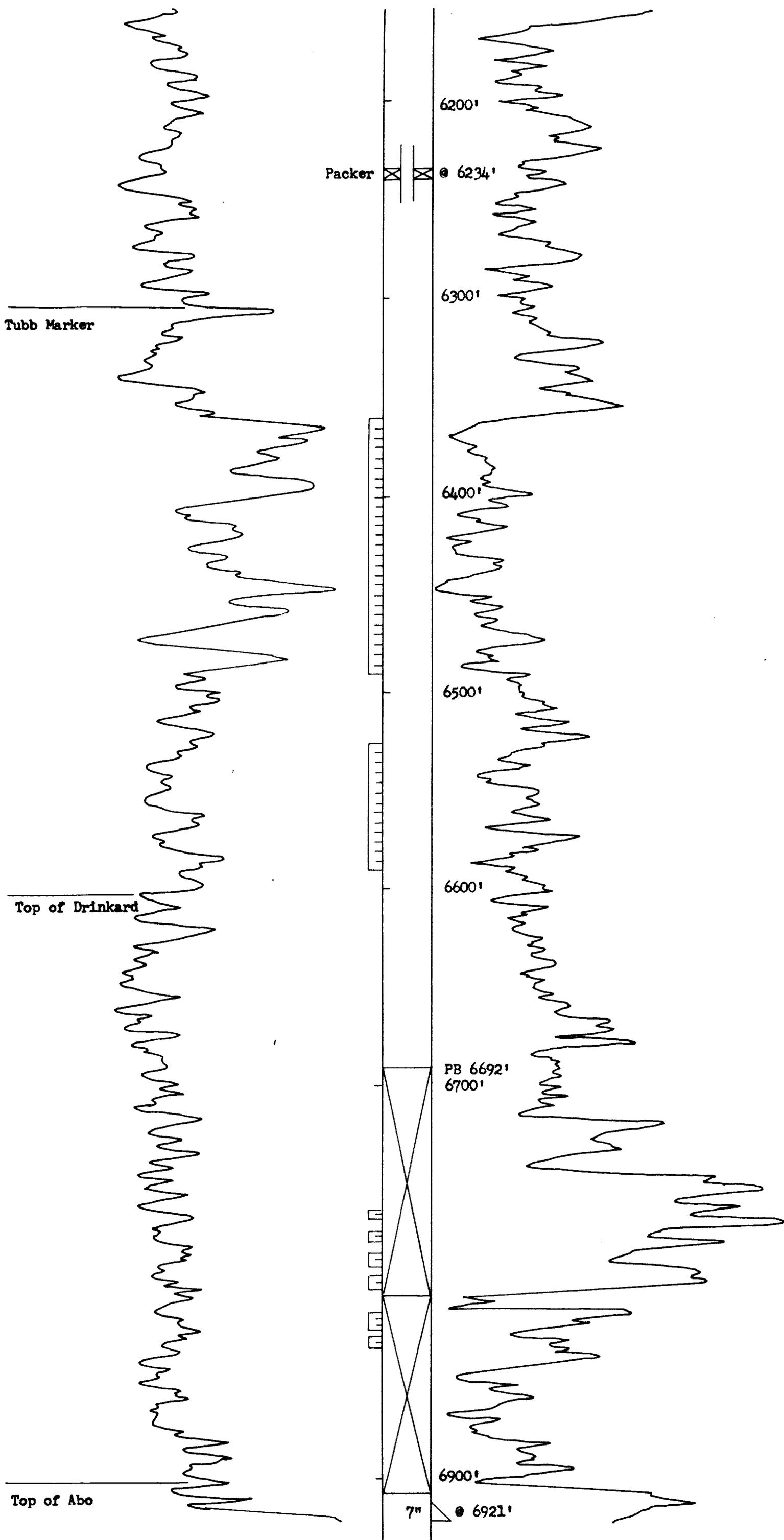
Dual Completion in Tubb, 2-11-57, for IP of 5810
