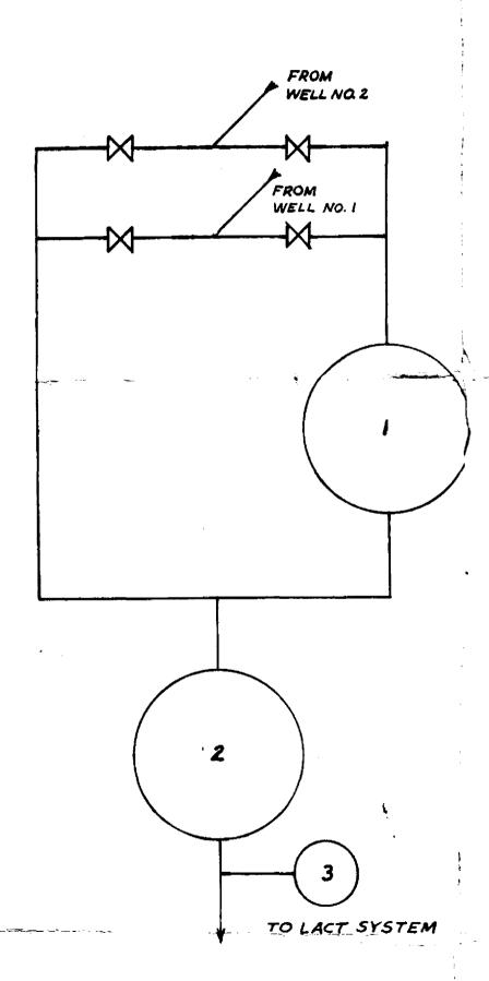
I METERING SEPARATOR (3 PHASE) FOR TESTING
