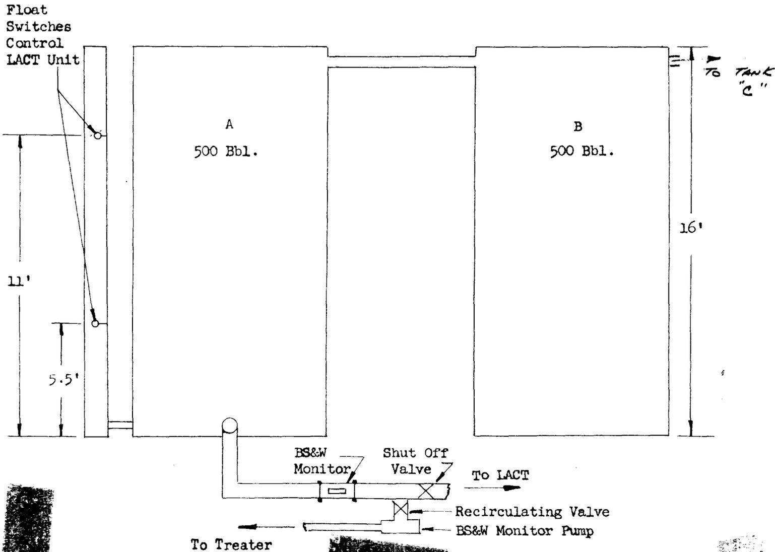
Reserve storage above top float switch in Tank "A" to top Tank "C" is 1177 bbls, at allowable rate of 749 BOPD, three wells @ 223 BOPD and one well at 80 BOPD, reserve storage time equals  $1177/749 = 1.57$  days or 37.6 hrs. Maximum time lease will go unattended is 18 hrs.
