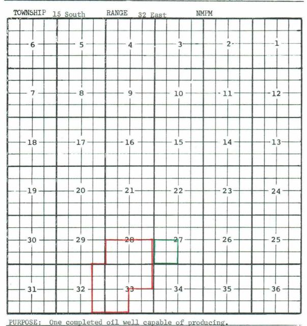
JOHN J. EISNER - Sinclair State #1 in Unit M of Section 27-15-32. Completed in Wolfcamp on November 14, 1962. Top of Perforations 10,084'.
