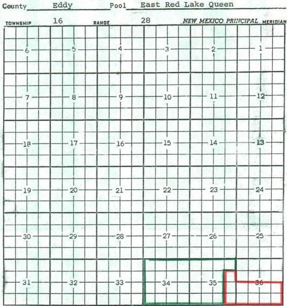
Purpose: To Combine two oil pools producing from the same formation, Queen, one oil well capable of producing and one gas well capable of producing. Kincaid & Watson Drlg. Co., Southern Union, Federal No. 7, in Unit K of Section 34:16-28. Completed in Queen, January 20, 1963. Top of perforation 1413'. Kincaid & Watson Drlg. Co., Trigg Fed. No. 1 in Unit E of Section 35-16-28. Completed in Queen, December 20, 1962. Top of perforations 1524' (Gas well)
