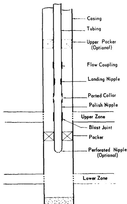
Fig. 1—Well properly equipped for multiple-completion choke assembly.
