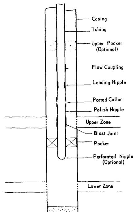
Fig. 1—Well properly equipped for multiple-completion choke assembly.
