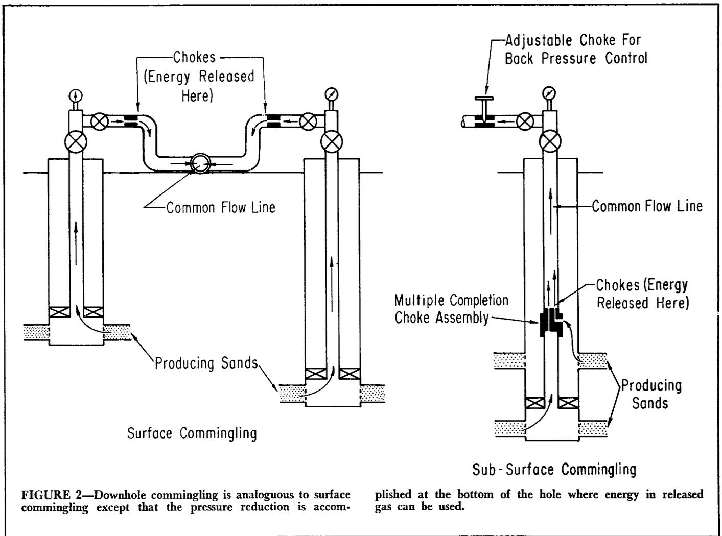
**FIGURE 2**—Downhole commingling is analogous to surface commingling except that the pressure reduction is accomplished at the bottom of the hole where energy in released gas can be used.
