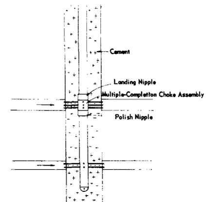
Fig. 10—One-string dual tubingless completion.
