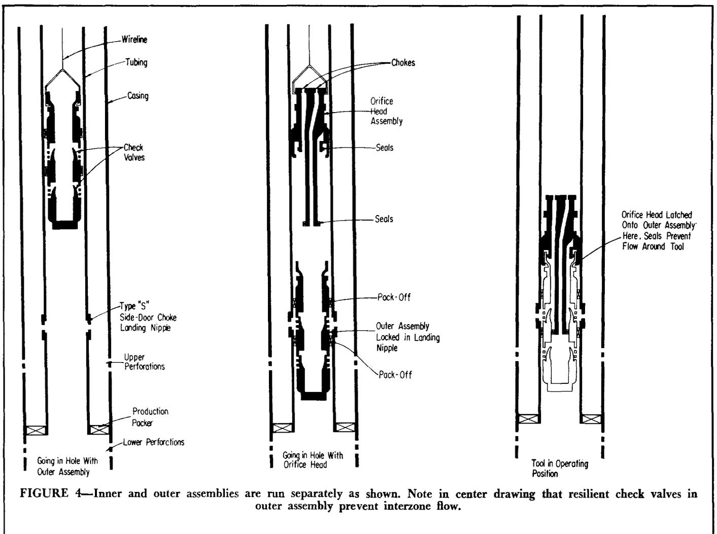
FIGURE 4—Inner and outer assemblies are run separately as shown. Note in center drawing that resilient check valves in outer assembly prevent interzone flow.
