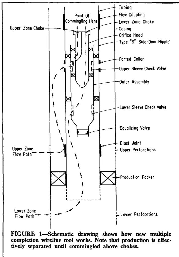
FIGURE 1—Schematic drawing shows how new multiple completion wireline tool works. Note that production is effectively separated until commingled above chokes.
