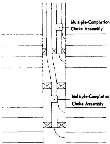
Fig. 5—Two-string quadruple completion.
