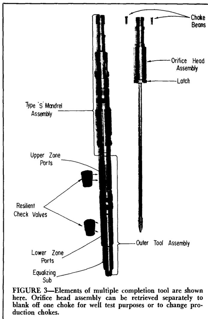
FIGURE 3—Elements of multiple completion tool are shown here. Orifice head assembly can be retrieved separately to blank off one choke for well test purposes or to change production chokes.
