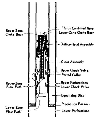
Fig. 3—Schematic drawing showing operation of multiple-completion choke assembly.
