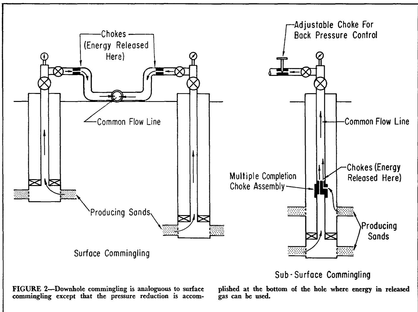
FIGURE 2—Downhole commingling is analogous to surface commingling except that the pressure reduction is accom-
