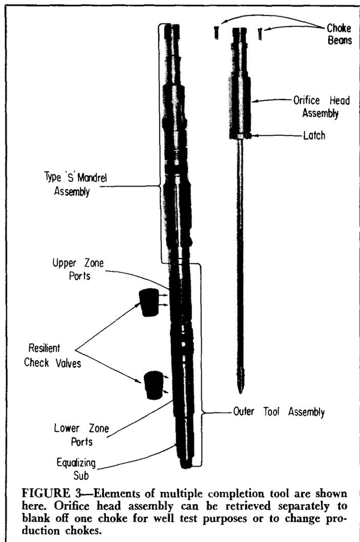
FIGURE 3—Elements of multiple completion tool are shown here. Orifice head assembly can be retrieved separately to blank off one choke for well test purposes or to change production chokes.
