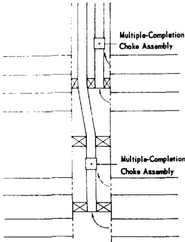
Fig. 5—Two-string quadruple completion.
