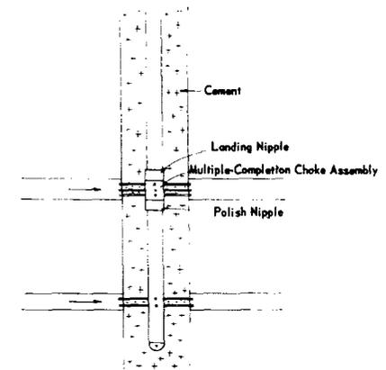
Fig. 10—One-string dual tubingless completion.
