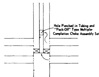
Fig. 9—Method of installing multiple-completion choke assembly in well not originally equipped with side-door choke landing nipple.
