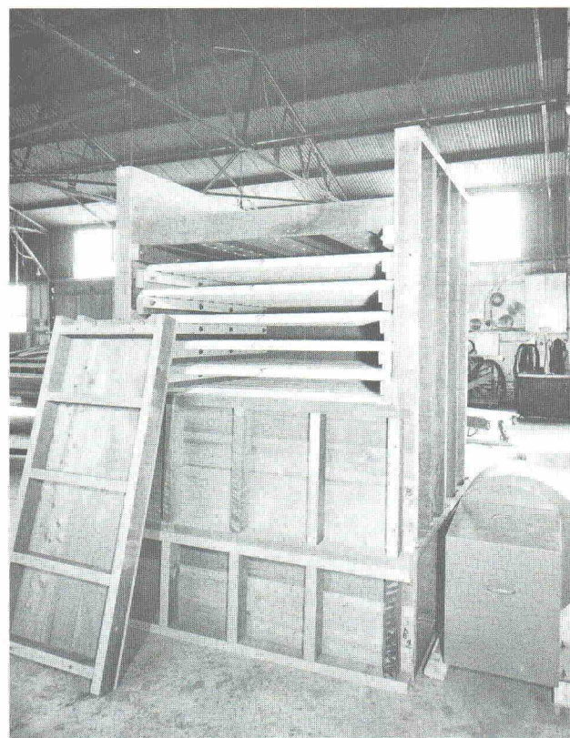
Small National Redwood Forced Draft Aerator with side panel removed. Note the Splash Baffles which slide out for ease of cleaning.
