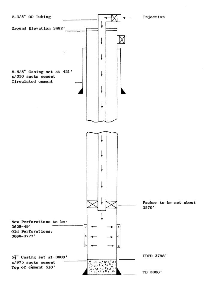
Schematic Drawing of Injection Well
