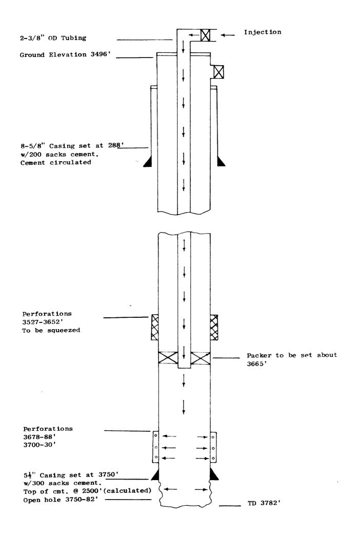
Schematic Drawing of Injection Well
