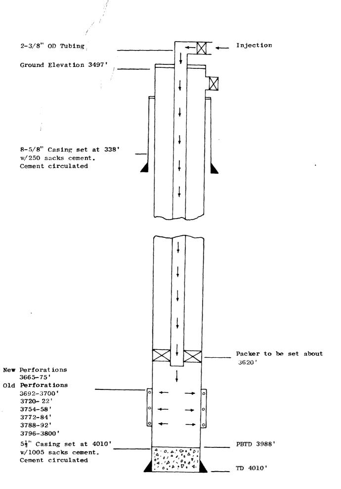
Schematic Drawing of Injection Well
