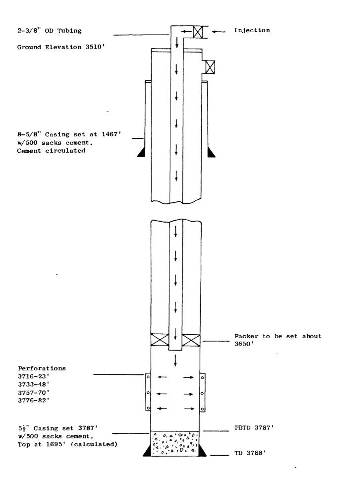
Schematic Drawing of Injection Well Unit Well No. 13 (ARCo Mattie Shipley No. 4) 660' FSL & 660' FWL Section 27, T-22S, R-36E
