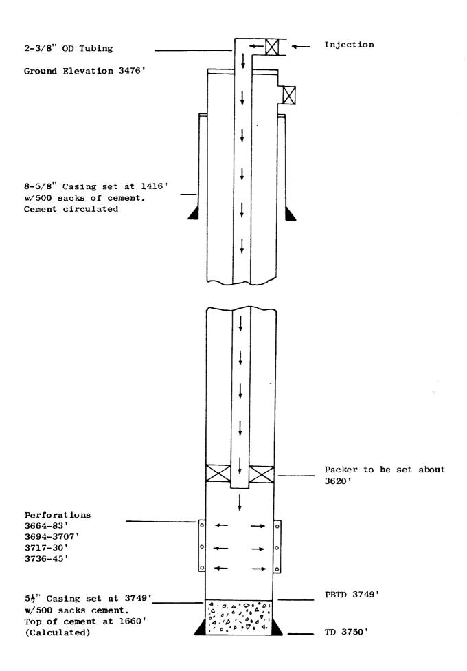
Schematic Drawing of Injection Well Unit Well No. 23 (ARCo C. Jones No. 9) 1980' FNL & 660' FWL Section 34, T-22S, R-36E Lea County, New Mexico
