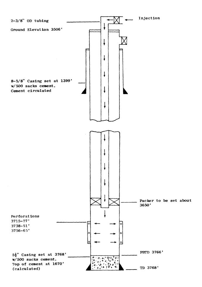
Schematic Drawing of Injection Well
