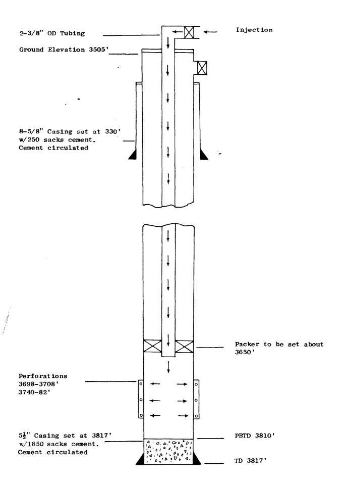
Schematic Drawing of Injection Well
