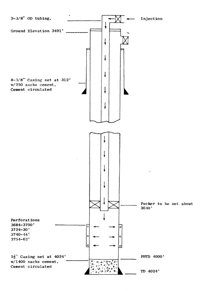
Schematic Drawing of Injection Well
