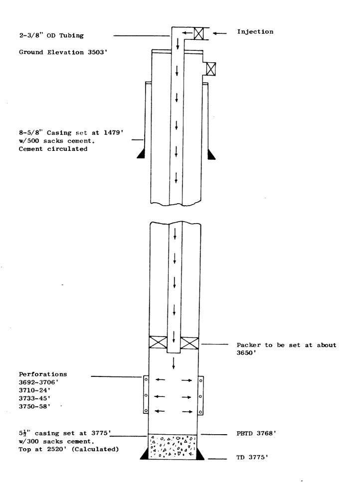
Schematic Drawing of Injection Well
