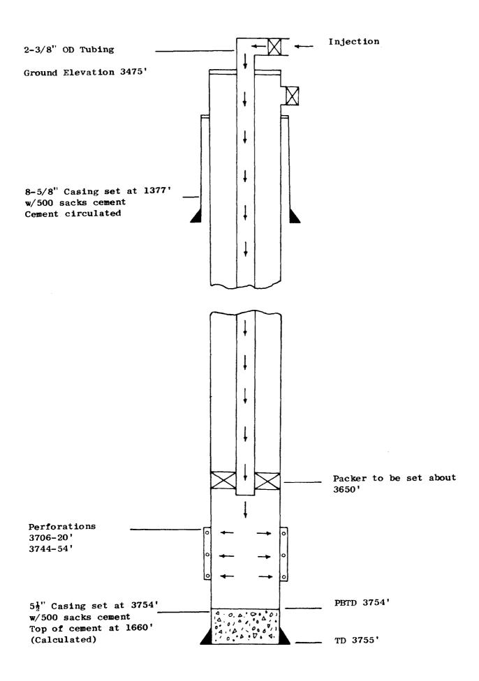
Schematic Drawing of Injection Well
