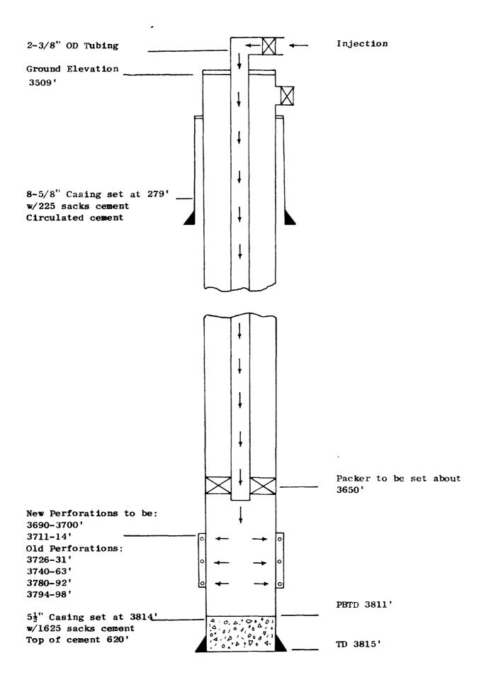
Schematic Drawing of Injection Well
