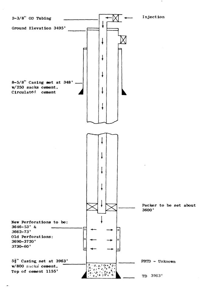
Schematic Drawing of Injection Well
