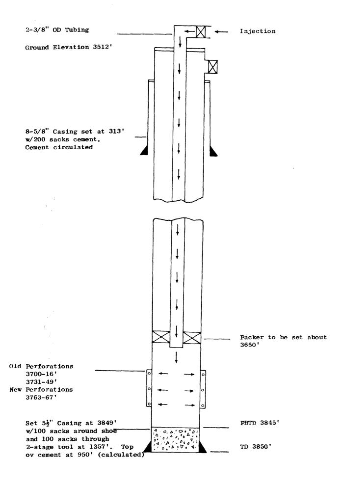
Schematic Drawing of Injection Well
