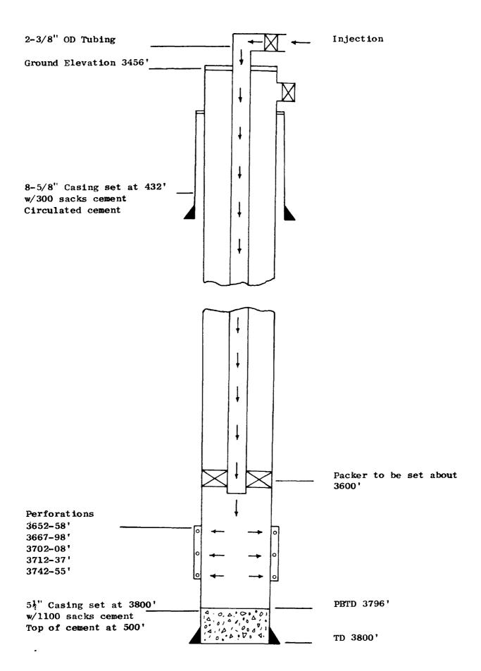
Schematic Drawing of Injection Well
