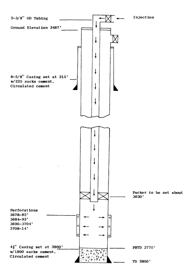
Schematic Drawing of Injection Well
