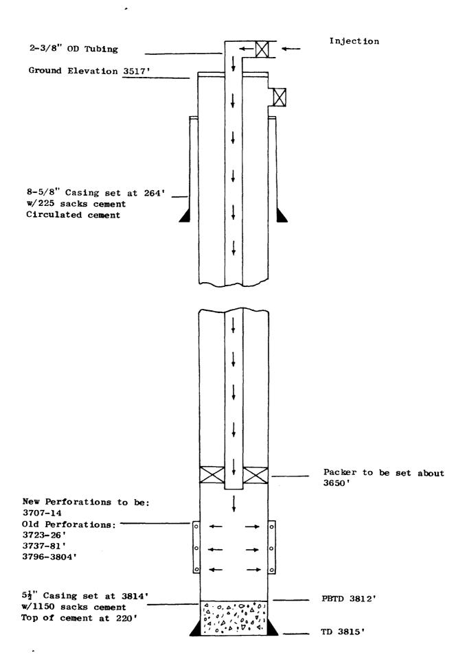
Schematic Drawing of Injection Well
