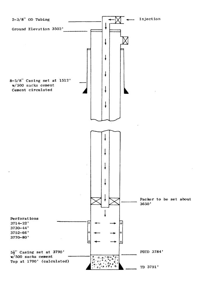
Schematic Drawing of Injection Well
