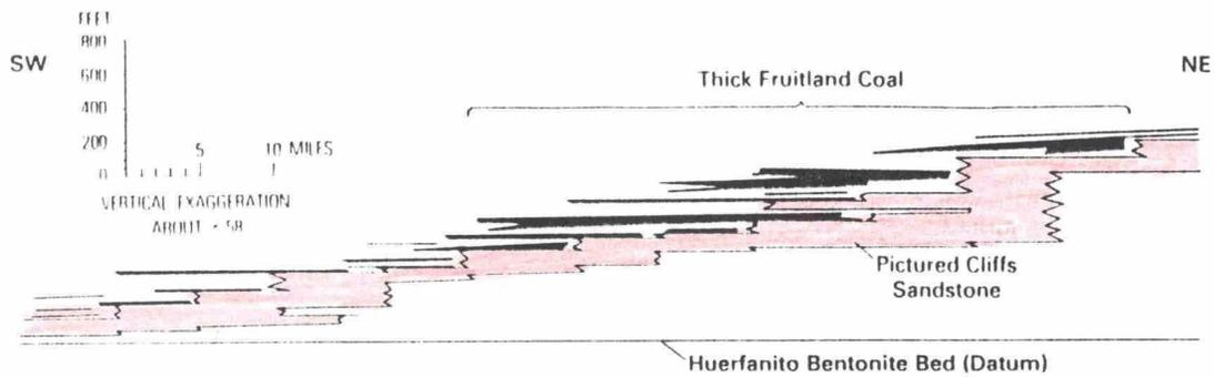
Northeast-trending stratigraphic cross-section showing Fruitland Formation coal beds and underlying Pictured Cliffs Sandstone. This cross section is modified from section B-B' of figure 8; coal bed thicknesses are from plate 3 of Fassett and Hinds (1971)
