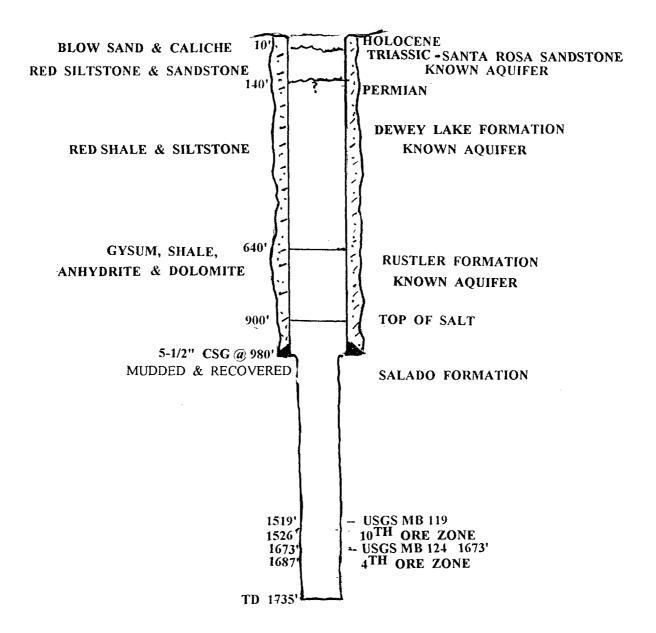
DRILLED WITH ROCK BIT TO 980', SET 5-1/2" CASING AT 980' RECOVERED ALL, CORED FROM 980' TO TOTAL DEPTH OF 1735' TD 1735' SET CEMENT PLUGS 0 - 10', 640 - 880', 900 - 1735'
