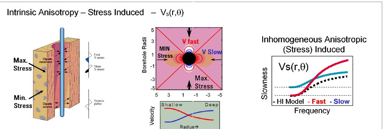
Shear velocity is a function of radius and angle, with the slowest shear velocity in the direction of minimum stress. On a dispersion plot, this is characterized as a crossover of the fast and slow shear as frequency increases.
